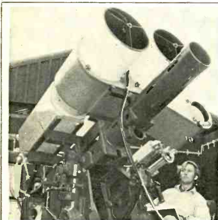
LOOKS LIKE A HOWITZER? Don't be too surprised—it's mounted on what was formerly an artillery piece. One of the large barrels is a laser transmitter—the other an optical camera.
