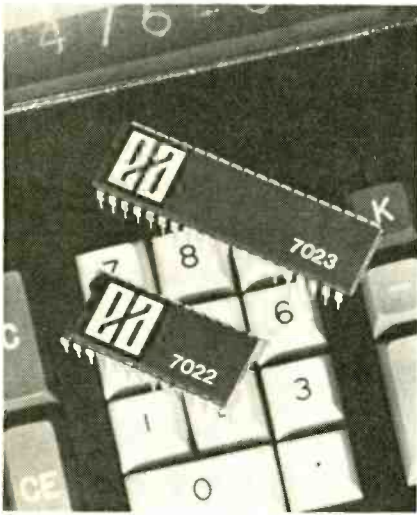
FIG. 7—MOS/LSI CALCULATOR circuit IC's introduced by Electronic Arrays, Inc.
